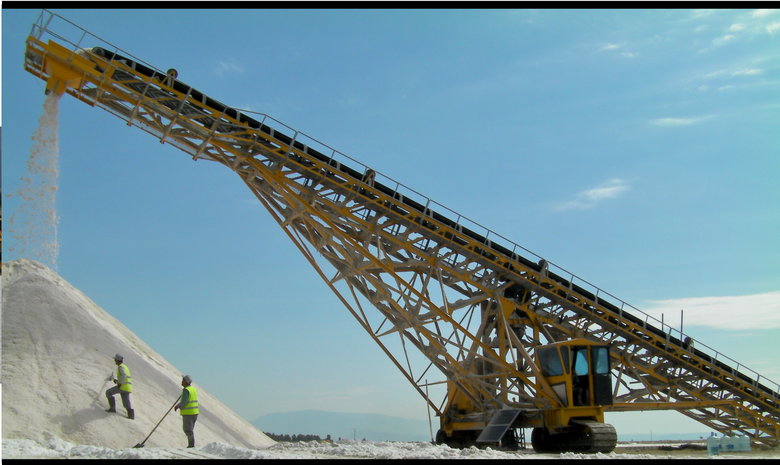
4 Track Stacker, designed to operate at various sites with collapsible mast for driving between sites. The tail of the stacker spans brine / bitterns channels.
