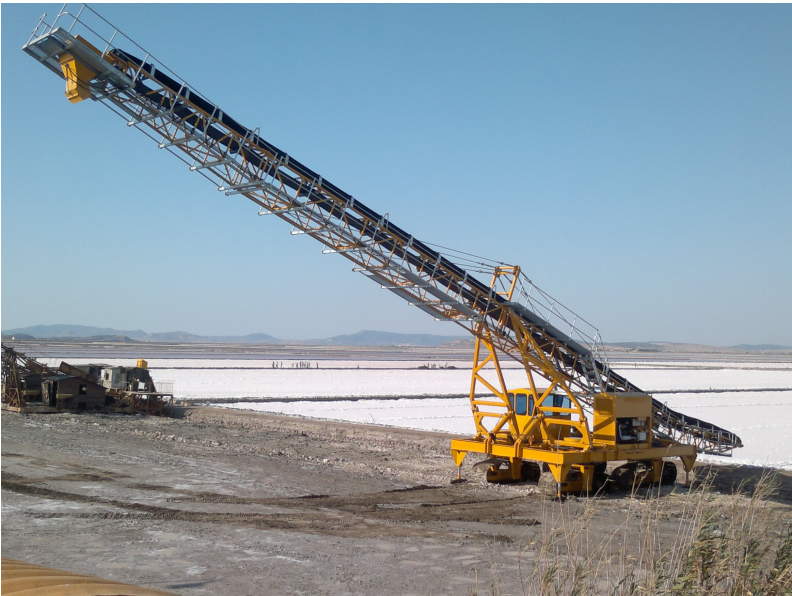
4 Track Stacker, designed to operate at various sites with collapsible mast for driving between sites. The tail of the stacker spans brine / bitterns channels.
